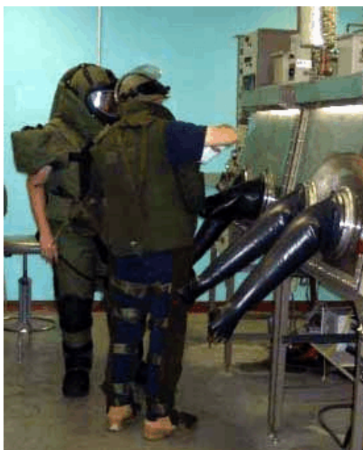
Cleanup personnel in bomb suits discuss decontamination of glove box involved in explosion. (Photo courtesy of Michigan Tech University.)
